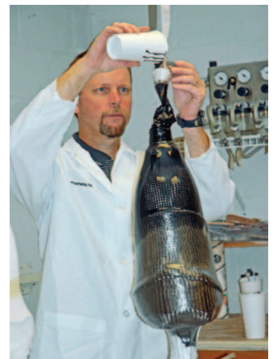
Adding catalyst-pigment mixture to activate socket lamination.
